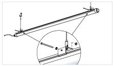
Attach both brackets to the Vapor Tight fixture. Secure brackets to fixture by using included anti-spread hardware. If needed, adjust wires until fixture is level. For Vapor Tight wiring, please refer to the installation instructions of Vapor Tight.
