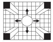
Four way intersections are the most common application for the domes. The ratio of viewing distance is estimated at one foot of viewing distance for each inch of dome diameter. In a warehouse setting, a wider viewing distance would help provide a safer view due to increased vehicle speed. The dome should be suspended as low as possible, yet taking into consideration elevated material activity. Available with Hardboard Back.
