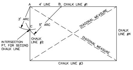
measurements from corner to corner. Diagonal measurement should be within 1/8" of each other to ensure the building is in square.
