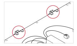
8. Insert the panel hangers into the frame details, (anglein and center). This will allow the panel to hang freely, and facilitate electrical hook-ups.
