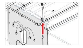
11. Locate the panel hooks (2) on the LED Flat Panel Retrofit and rotate them to the open or install position.
