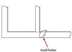
2. Locate the stationary mounting tabs on the frame (2). Insert these tabs, on top of the grid ceiling "T" rail, and beneath the troffer.
