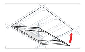
4. Rotate the mounting cams on the frame (2) to the engaged position. The mounting cams should be flush to the T-rail grid cams and be resting on top of drop ceiling "T" grid. The frame is now installed. Inspect installed frame to ensure the gaps from side to side are even.
