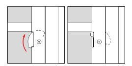
Attach seismic safety cables using self-tapping screws (2 ea. provided) as needed. Clip to holes in frame. Screw tabs on other end of cables to inside of troffer.
