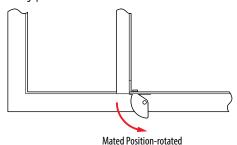
1. Ensure that the rotating mounting cams (2) on the frame are in the open or install position.
