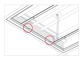
7. Locate the two panel hangers on the side edge of the retrofit panel (one shown) opposite the panel hooks.
