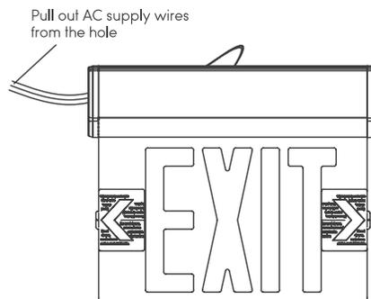
5. Now connect the wires. If you're using 120V AC, connect the black and white wires to the building wires. If you're using 277V AC, connect the red and white wires to the building wires. 6. Attach the mounting bracket to the crossbar with the PM4\*20 screws. 7. If the chevrons are needed, PLEASE keep them and tear off the instruction stickers on the panel. If not needed, tear off all the stickers on the panel.
