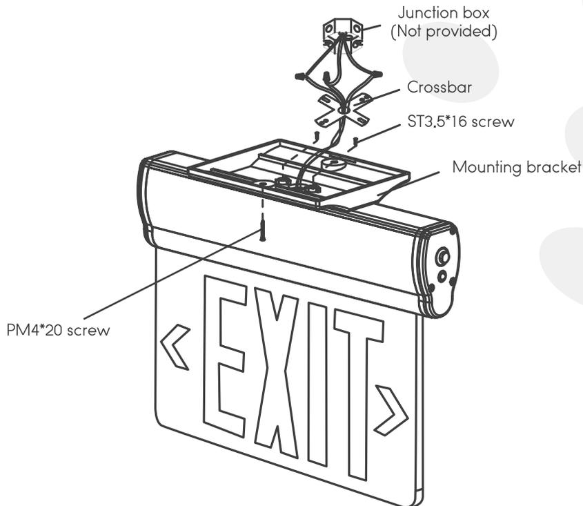
5. Now connect the wires. If you're using 120V AC, connect the black and white wires to the building wires. If you're using 277V AC, connect the red and white wires to the building wires.
