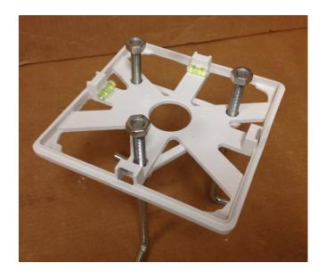
This is the bottom base plate of the Bollard. Loosen the (4) set screws from the bottom of the Bollard and remove. Place over mounting bolts and tighten nuts. Postion Bollard housing over mounting plate and retighten set screws.
