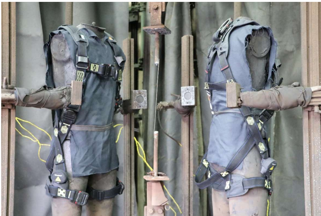
Figure 6.1: Sample set up before arc exposure.
