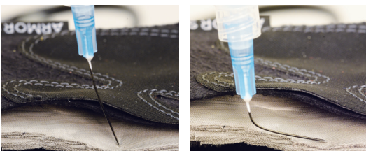
25 gauge needle buckling 25 gauge needle failure
