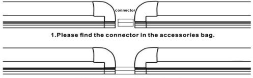
2. Plug the connector into the tube.
